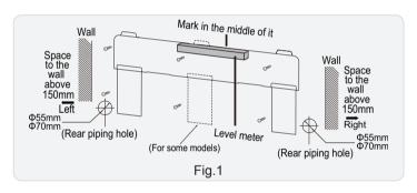
(2) Open a piping hole with the diameter of  $\Phi$ 55mm or  $\Phi$ 70mm on the selected outlet pipe position. In order to drain smoothly, slant the piping hole on the wall slightly downward to the outdoor side with the gradient of 5-10°.(As show in Fig.2)
